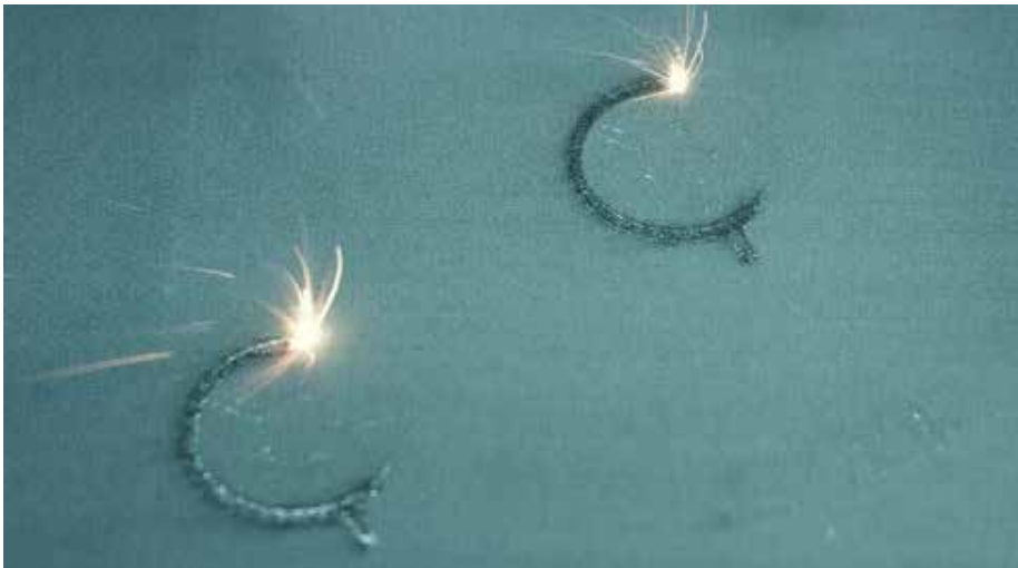
Image of laser powder bed fusion with two lasers during printing (note effluent from each melt pool).
