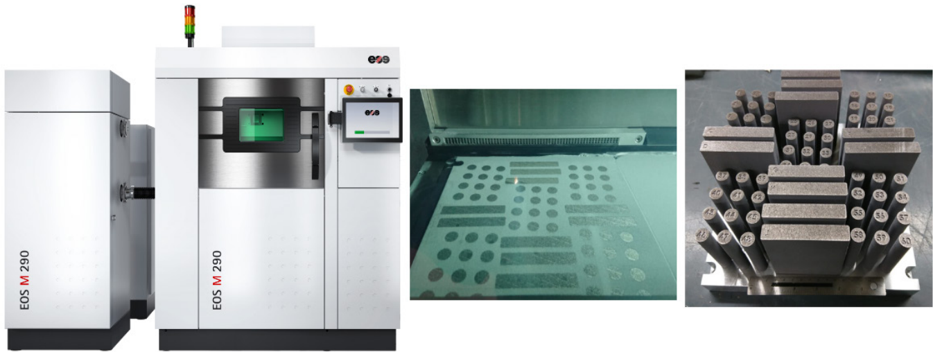
EOS M290 LPBF system printing samples with completed print.
