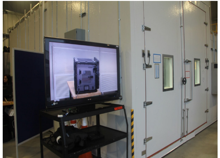
Craitor demonstrating print capabilities at -40°C during the OSD PoN Challenge
