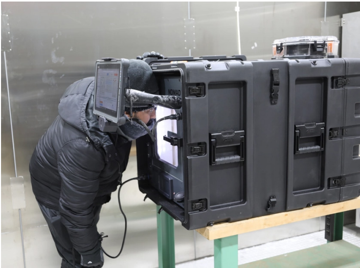
Craitor demonstrating print capabilities at -40°C during the OSD PoN Challenge
