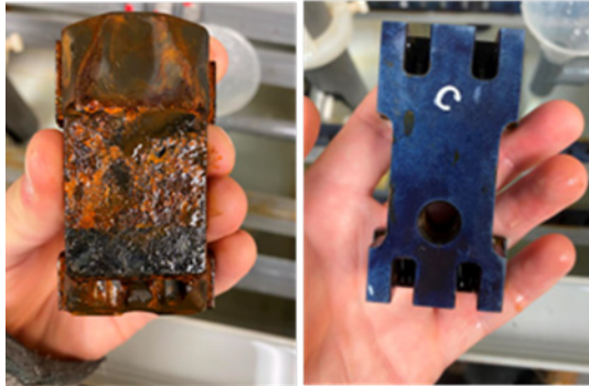
M197 Gatling gun bolt after 168-hour salt fog exposure with and without ANC cavitation and corrosion of AM stainless steel coupons with 3-hour and 6-hour ultrasonic cavitation.
