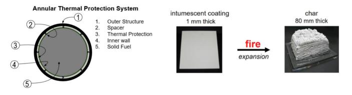
Massive insulation of intumescent coatings may reduce the temperatures that structural materials are exposed to and allow less exotic composites in solid rocket motor designs and high-temperature applications.
