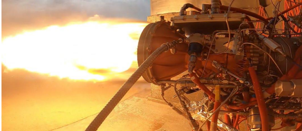
Hotfire testing GrCop-42 Thrust Chamber Assembly (TCA) on the vacuum variant of the Hadley liquid rocket engine.
