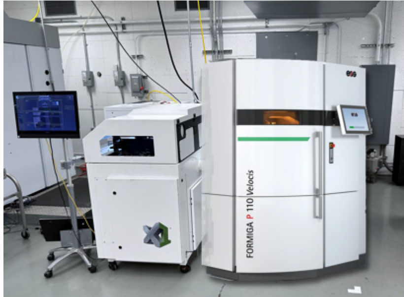
EOS P110 Polymer Laser Sintering Machine used in cold metal fusion printing process
