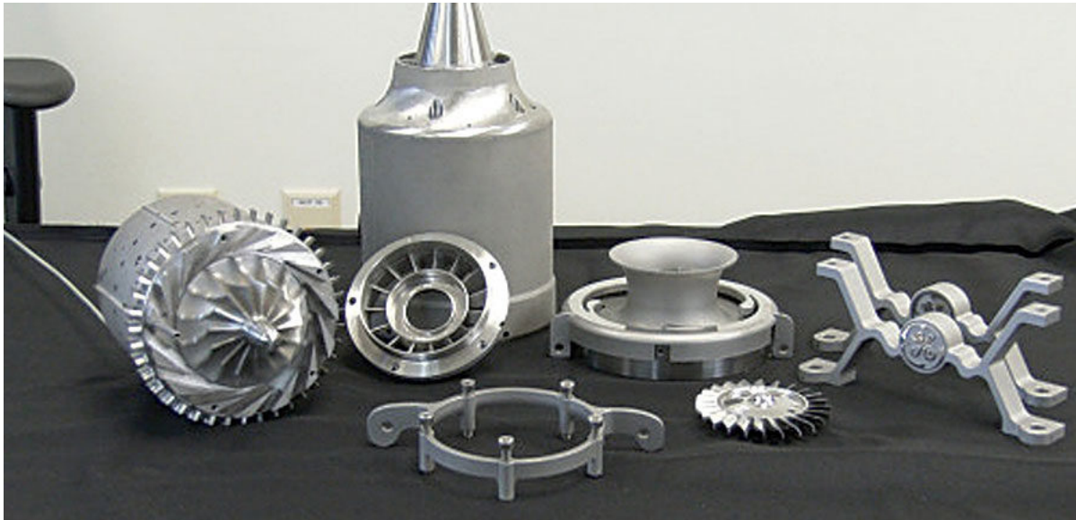
Functional Jet Engine Parts Built Using AM (GE Aerospace)
