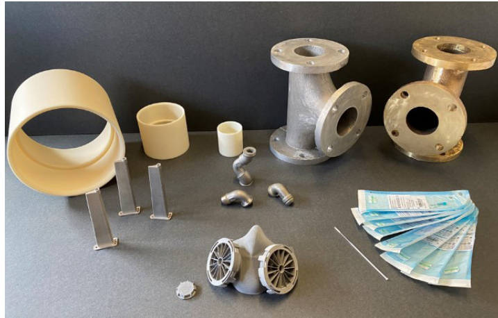
Parts additively manufactured by ecosystem suppliers during Scenario Execution
