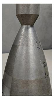
Rocket nozzle printed with multiple lasers, each utilizing the same parameters. Variance in surface finish between lasers is evident.
