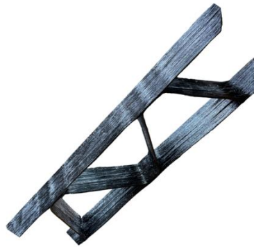
Figure 2: Carry-through structural member prototype taking into account manufacturing constraints of continuous fiber additive manufacturing.
