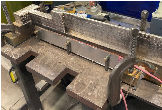
Photographs depicting arc directed energy deposition standard qualification builds produced for (a) single sided nickel aluminum bronze alloy and (b) double sided high strength steel alloy with integral build platforms.
