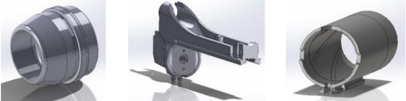
CAD renders of each of the 3 specific parts printed: projectiles, receivers, and barrels.
