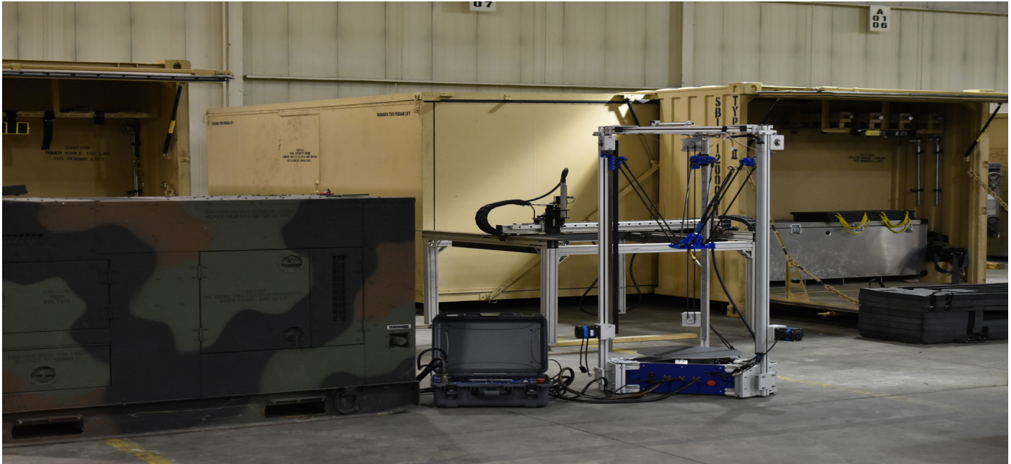
Prototype expeditionary wire-arc additive manufacturing system shown with an Army MWMSS used for forward operating bases.
