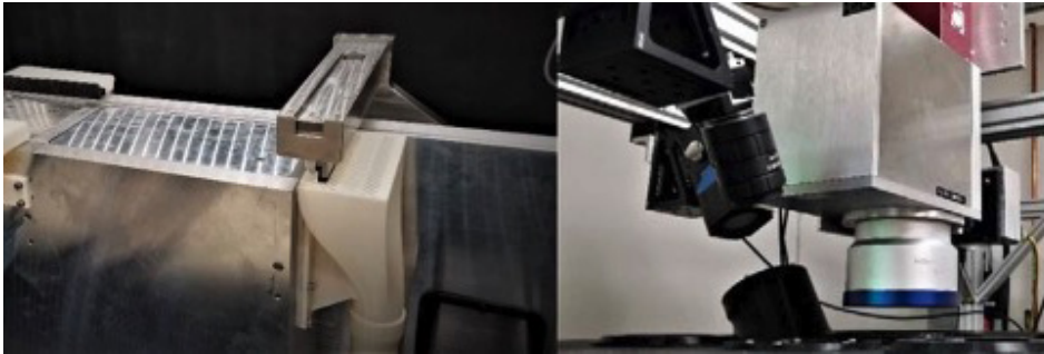
DART SLM powder cell at UDRI (left) and in-situ sensors installed on UDRI's DART SLM (right).
