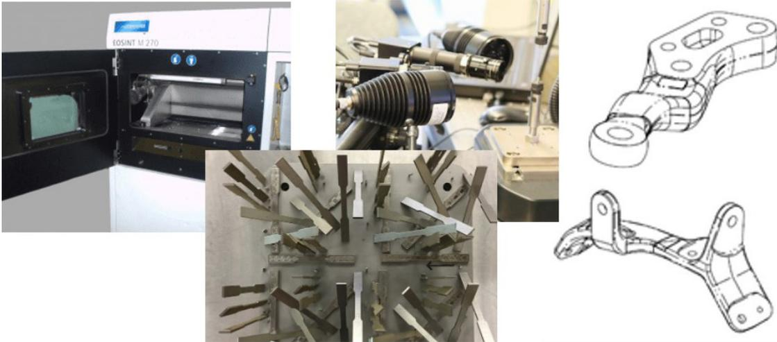
*This project involves comparing test specimens from multiple machines and multiple locations, as well as optimizing the geometry of some "real world" parts for additive manufacturing.*
