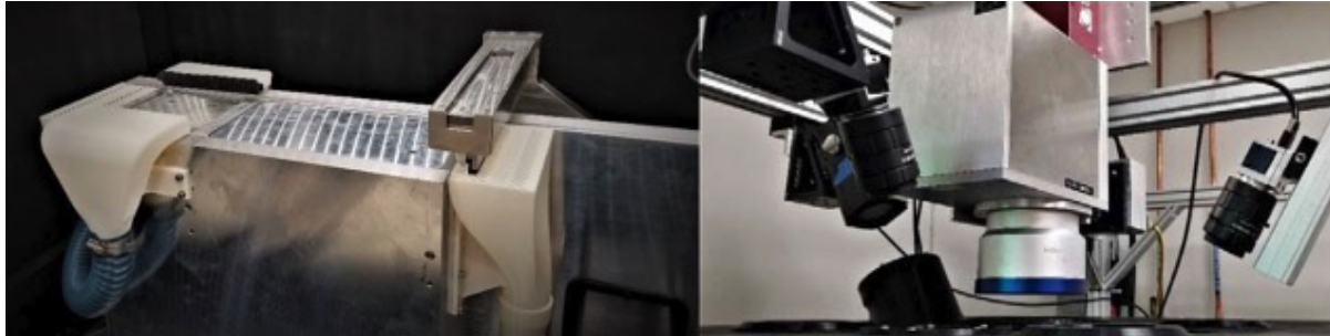
DART SLM powder cell at UDRI (left) and in-situ sensors installed on UDRI's DART SLM (right).
