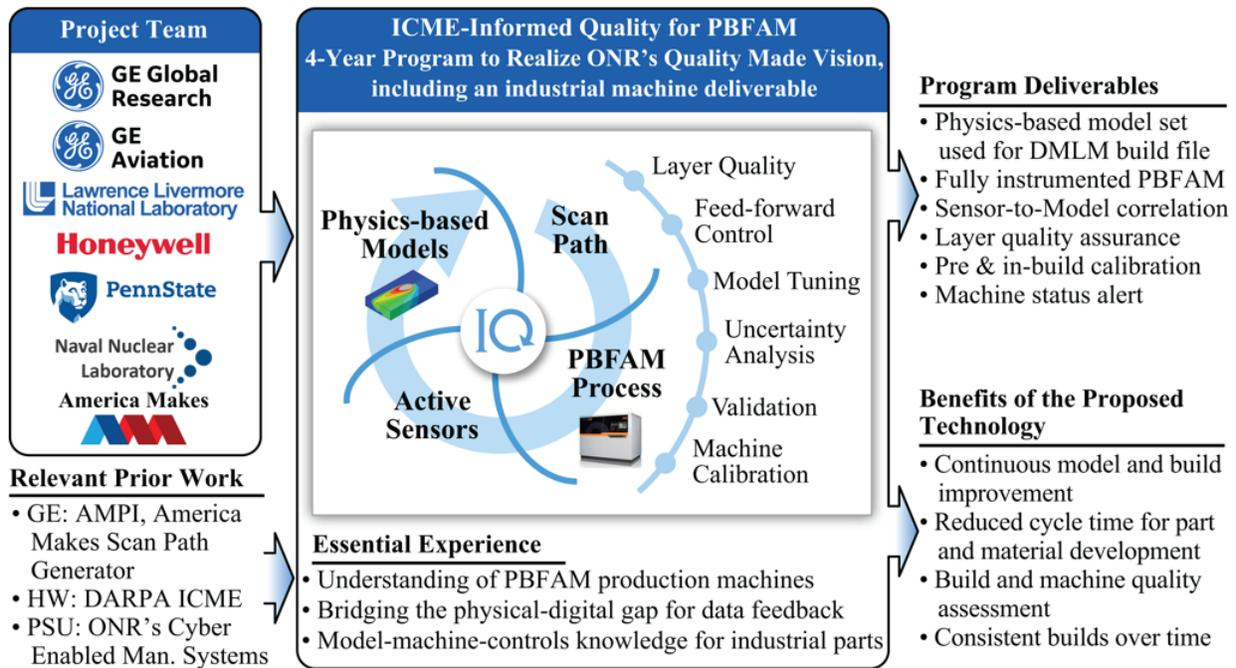
*An industrialized and intelligent metal powder bed fusion additive manufacturing system that links on-machine sensor output with physics-based models to provide greater process control over a complex part geometry.*
