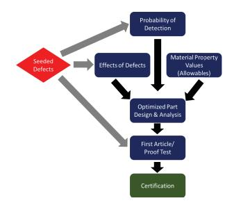
The ability to seed representative surrogate defects into otherwise nominal material can provide fundamental understanding of mechanical performance debits and critical flaw sizes necessary for LPBF process and nickel alloy 718 material qualification.
