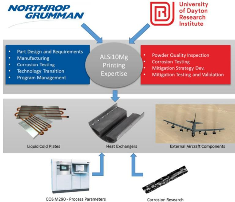
*Liquid cold plates, heat exchangers, and external aircraft components are of interest for this corrosion investigation by the team composed of Northrop Grumman Systems Corporation (NGSC) and University of Dayton Research Institute (UDRI).*
