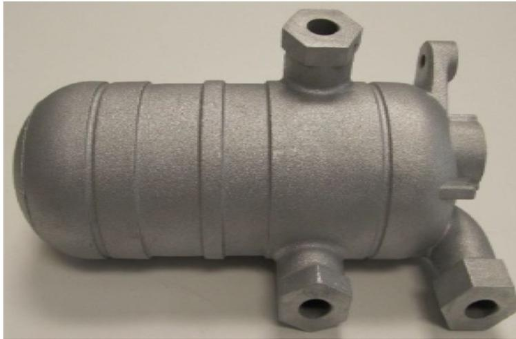
*Generic fuel cooled oil cooler which features thin wall channels (interior not shown) within a shell volume of fuel. Fuel is an active cooling medium for the oil and the preheated fuel improves engine efficiency.*
