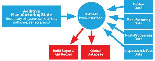
CIMP-3D created a Data Management System for Additive Manufacturing (DMSAM) to capture all data and processing configurations associated with the entire additive manufacturing process. DMSAM uses a natural progression of data entry during the planning, manufacturing, and inspection stages, adding utility based on the function of each stage.
