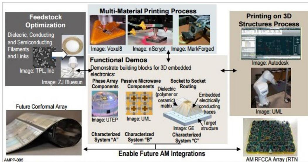
Interactions across the 3D printing value chain from feedstock optimization to equipment and software are all required to optimize the multi-material printing process for 3D embedded electronics.
