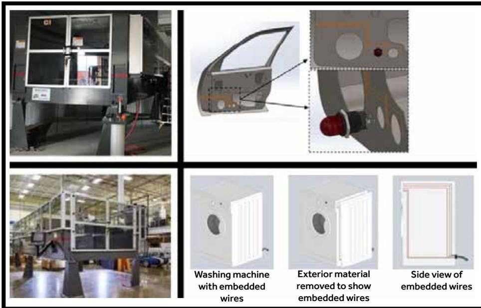
*BAAM + wire embedding allows for wire embedding to be 3D printed directly into structures such as car doors to supply power to lights and speakers, or in washing machine side panels to provide wiring to the control panel.*
