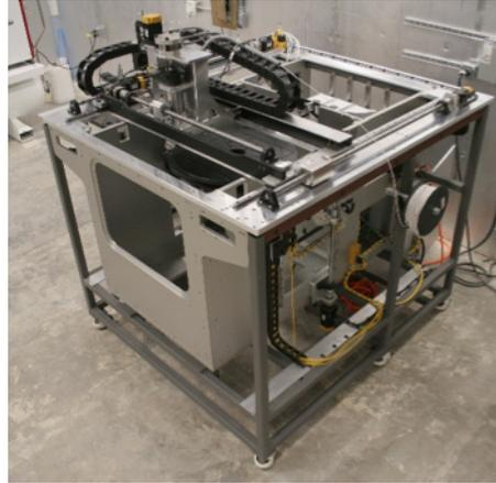
*A five-axis motion system, collectively referred to as Multi<sup>3D</sup> manufacturing, provides spatial control of material and functionality within a single enclosure containing a suite of complementary additive and subtractive manufacturing processes.*
