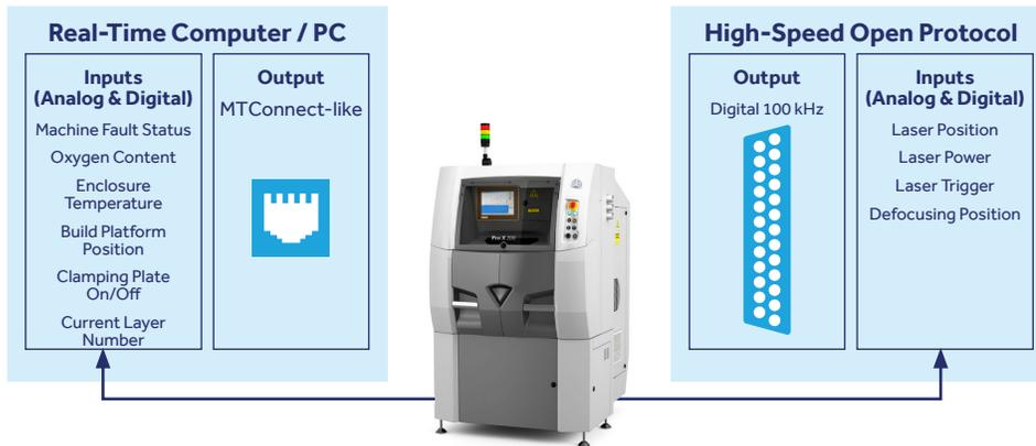
*The ability to read and output real-time, high-speed measurements and output scanner positions and laser time was demonstrated. Direct comparison between build plan and high-speed measured data have also been demonstrated using standard coupons.*
