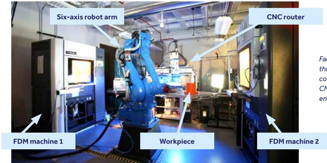
*Fabrication of electronic systems through a multi-technology system combining material extrusion, CNC routing, direct-write, and wire embedding capabilities.*
