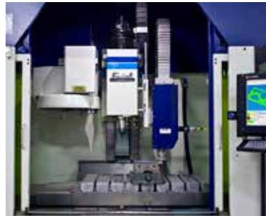
*The hybrid concept incorporates additive manufacturing (AM) on familiar CNC platforms, expanding the use of AM by making it available on a conventional machine tool.*
